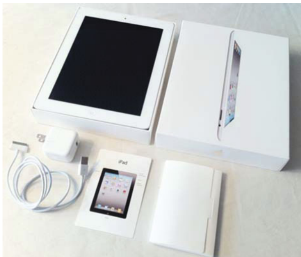
Figure 1–2. There’s not much inside the iPad box: the iPad, a Dock Connector to USB Cable, a 10-watt AC adapter, and some simple documentation.
