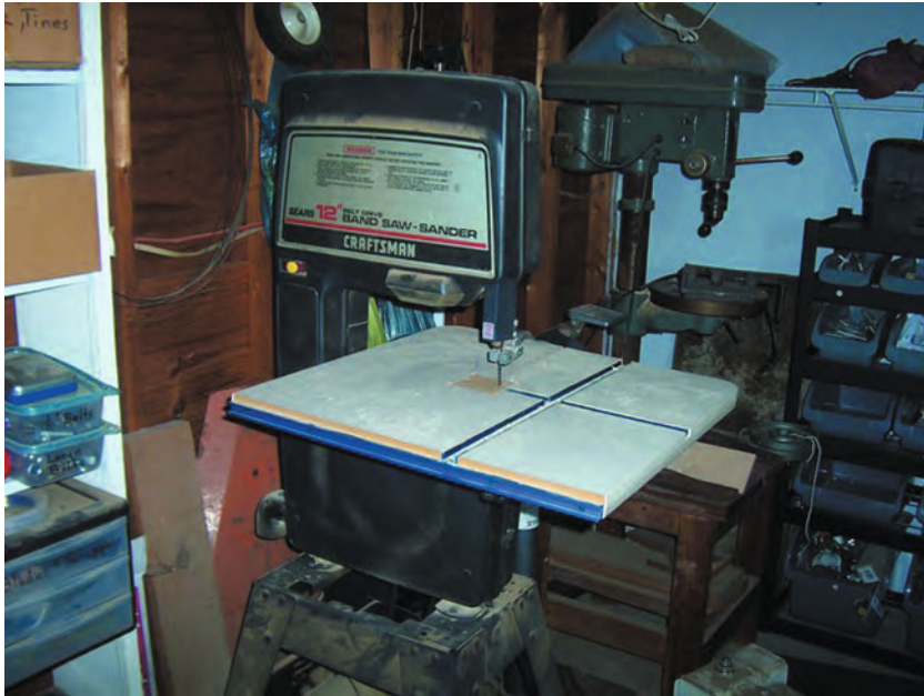
Figure 2-4. A bandsaw or scroll saw can be useful for cutting ninety degree corners.
