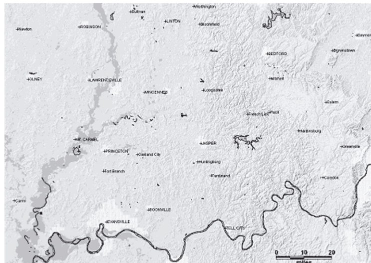
Fig. 4. Rapid response inundation map of the Wabash Valley (left portion of map) based on MODIS data. The light grey tones show areas flooded, the dark grey outline encloses water imaged by MODIS during non-flooded conditions. Shaded relief base material was generated from NASA Shuttle Radar Topography Mission (SRTM) topographic data
