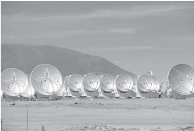
Figure 1.3. The Atacama large millimeter/sub-millimeter array (ALMA) interferometer in Chile. (Credit: ALMA (ESO-NAOJ-NRAO), J. Guarda.)
