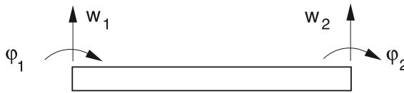
Figure 2-14: Alternative representation of the deflections
