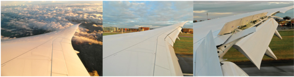
Figure 1.2 Three wing geometries packaged into one and able to morph from one to another: the trailing edge of the wing of a Boeing 787-8 airliner in (from left to right) cruising flight, final approach and touch-down (photographs by A. Sóbester).
