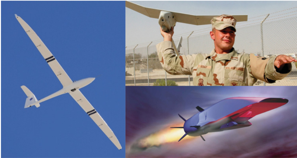
Figure 1.1 Three unmanned air vehicles (UAVs), three main design drivers: NASA Towed Glider Air-Launch Concept (left, NASA image) – long endurance at low speeds; AeroVironment RQ-11 Raven (top right, USAF image) – structural robustness to cope with battlefield conditions; Boeing X-51 (USAF image) – extremely high speed.
