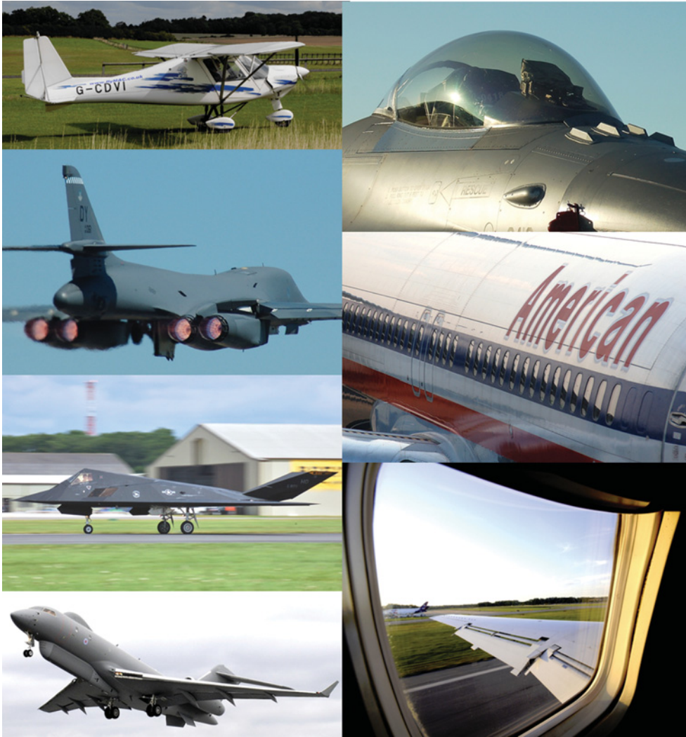
Figure 1.3 External (or outer mould line ) geometry – even within the realm of fixed-wing aircraft, the variety and sophistication of surface shapes poses a serious geometry modelling and optimal design challenge (photographs by A. Sóbester).
