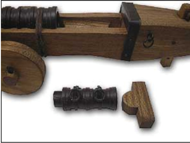
Figure 1.4 Showing active region of a breech-loaded cannon as used on the Mary Rose. Reproduced with permission from The Mary Rose Trust. © The Mary Rose Trust, 2014.
