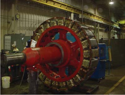
Figure 1.3 Photograph of a salient pole rotor for a large, low speed motor (Source: Photo courtesy Teco-Westinghouse).
