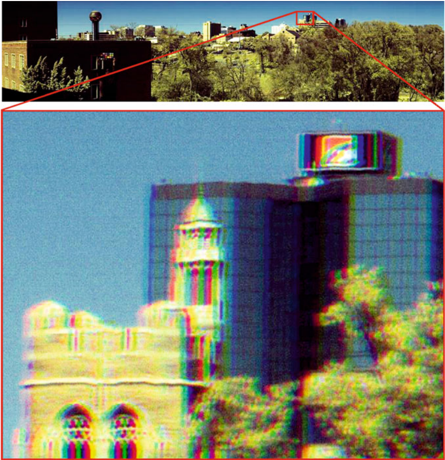
Fig. 4 Color misalignment in a multi-line CCD image
