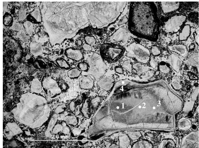
Fig. 8 Lethlekane (Botswana) diatreme zone KPK consisting of serpentine–chlorite pseudomorphs after olivine set in a chlorite–diopside interclast matrix. Back-scattered electron image. Numbers indicate analytical points (see Table 2)
