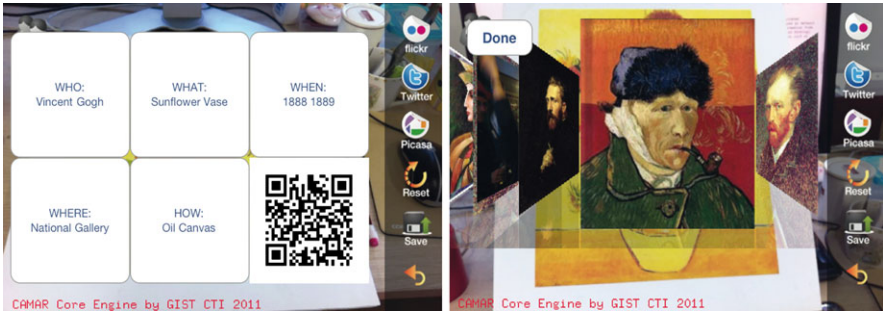
Fig. 1.18 Bar code identification of the object of interest and augmented reality output (from [238])
