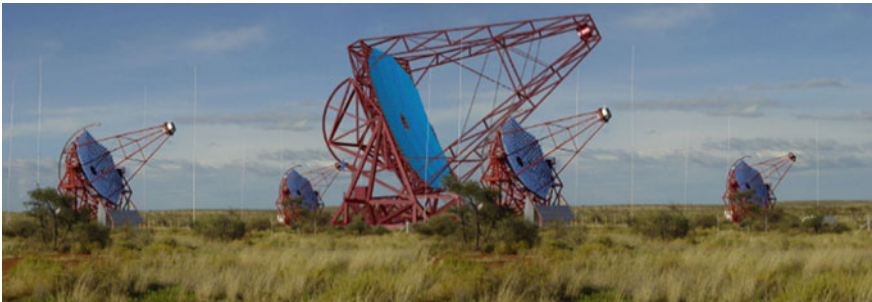
Fig. 4 The HESS system of four 13 m diameter Cherenkov telescopes. While this system has been operating in Namibia since 2003, the new 28 m diameter telescope is under construction (the picture in the center of the original HESS array is a photo montage)
