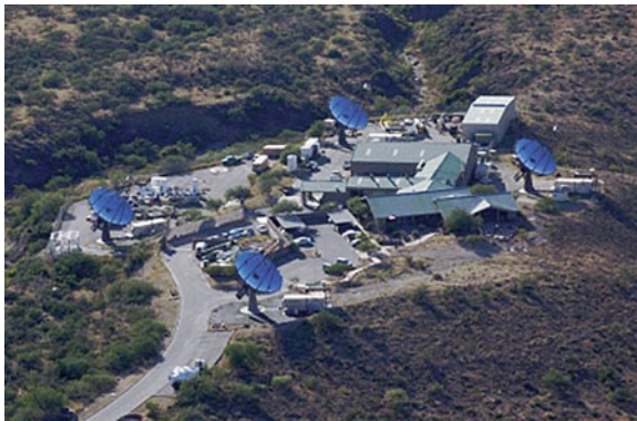
Fig. 6 The VERITAS system of four 12 m diameter Cherenkov telescopes located in southern Arizona
