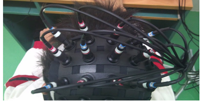
Fig. 2 Three illuminators and three detectors in arrangement result in 7 channels on each hemisphere where red optode illustrates illuminator and blue optode illustrates detector.
