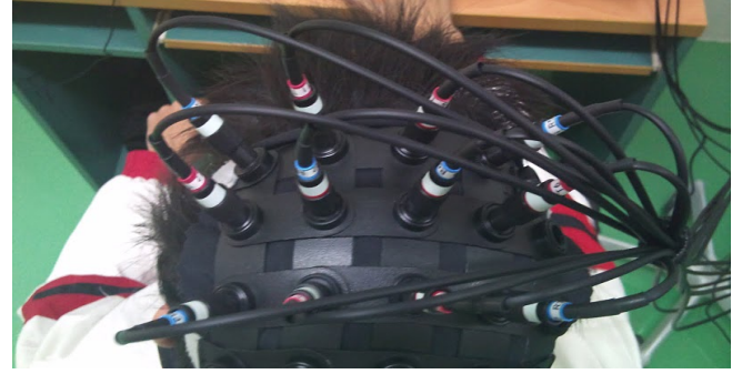
Fig. 2. Three illuminators and 3 detectors in arrangement result in 7 channels on each hemisphere where red optode illustrates illuminator and blue optode illustrates detector.
