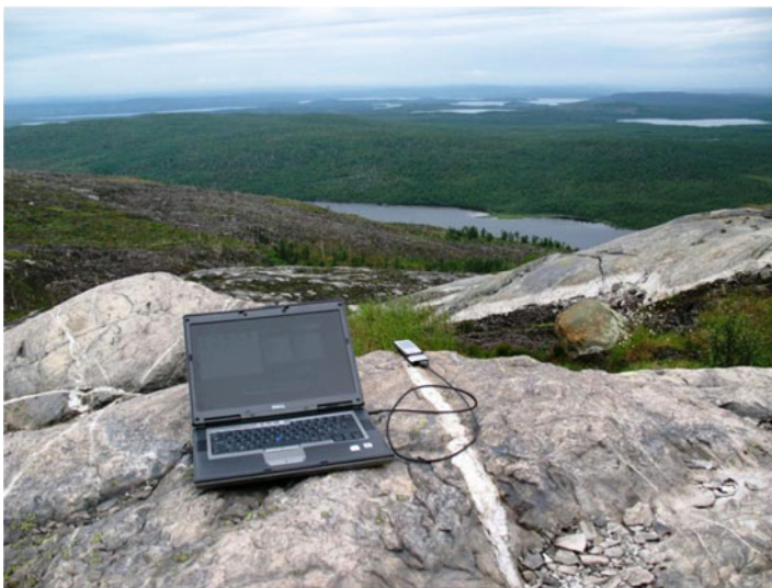
Fig. 5.3 To the left: The cell phone was used during the field expedition for the transfer of data from the FAR-DEEP DIS server installed on a standalone laptop to the central ICDP server in Potsdam (Photo from the hill top (best cell phone signal) in the Pechenga Greenstone Belt
