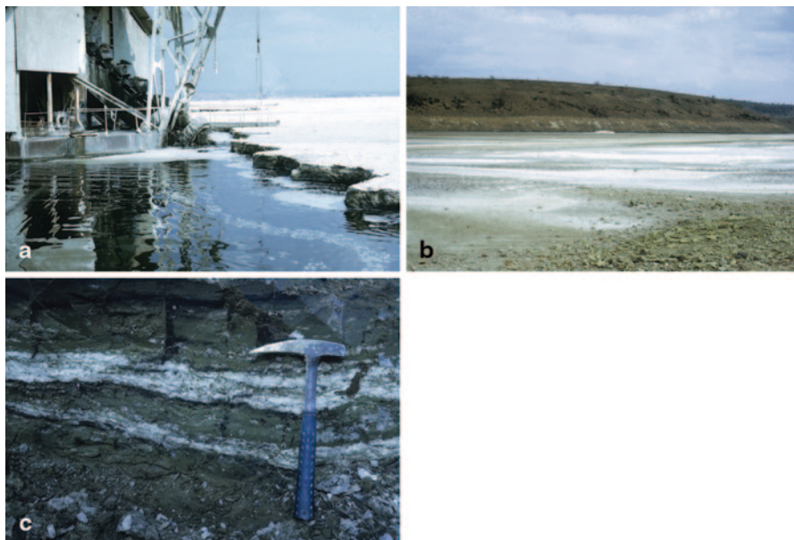
Fig. 1.8 (a) Modern trona mining operation at Lake Magadi, Kenya. The dredge is extracting the trona beds; if the dredge shut down, it would become trona-locked because the brine is saturated with trona. The trona beds are masses of trona crystals filled with brine. As the trona is mined, the brine flows out of the trona to form the “lake” upon which the dredge is floating. (b) Present-day Magadi mudflats with trona efflorescent crust. The 10,000-year high-stand shoreline of Lake Magadi (High Magadi Beds) is in the background. (c) High Magadi Beds associated with the high-stand shoreline shown in (b). The sediments are organic-rich (black) with fish fossils. The white layers consist of magadiite, a hydrous sodium silicate that, with time, reacts to Magadi-type cherts. Carbon-14 dating suggests that these organic-rich sediments are approximately 10,000 years old. Therefore, over the past 10,000 years the lake evolved from a relatively fresh lake supporting a fish population to a saline, alkaline lake precipitating trona
