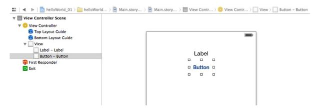
Figure 2-11. Placing the "Button" control on the view
