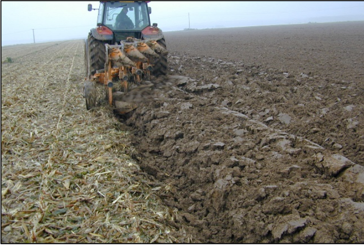
Figure 1.2. Mechanized plowing, Grignon plateau, 2002. Crop residues (corn) located on the surface of the soil are buried by tillage (photo credit: C. Coutadeur)
