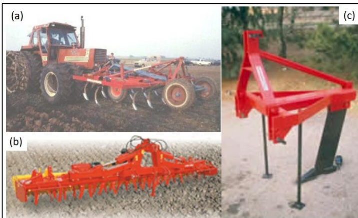
Figure 1.9. Tillage tools: (a) front cultivator; (b) rotary harrow; (c) subsoiler (photo credits: Pottinger, Quivogne). For a color version of this figure, see www.iste.co.uk/coquet/agricultural.zip
