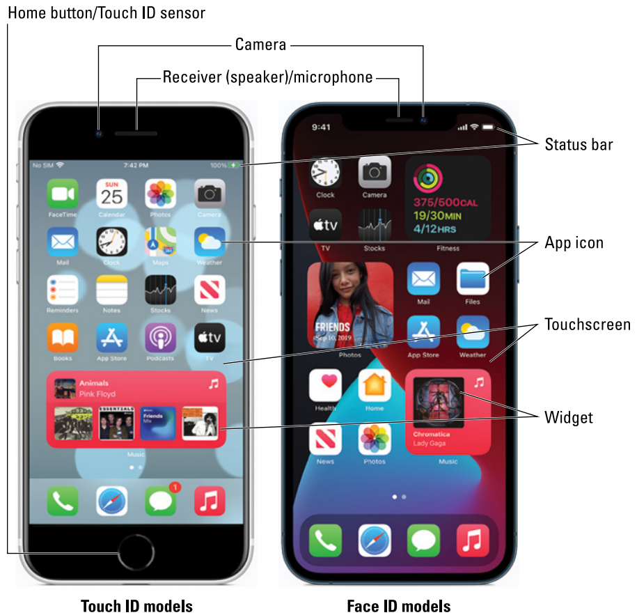
FIGURE 1-1: Touch ID iPhone models (left) have a Home button, whereas Face ID iPhone models do not.
