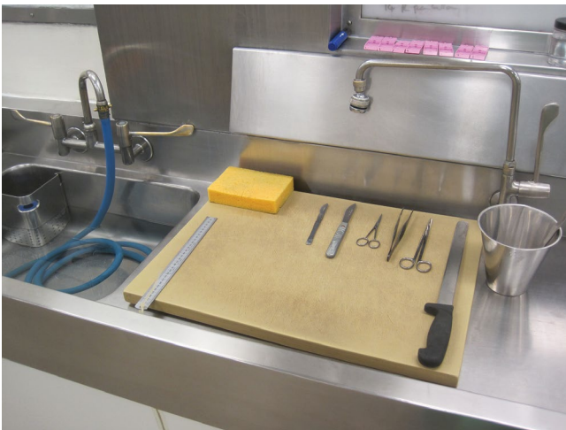
Fig. 1.25 The pathologist dissection bench is shown with the essential instruments for examination. These include a large or long knife, scissors, small and large scalpels, forceps, sponge, and ruler. Also needed are local access to running water, a measuring jug and histology cassettes
