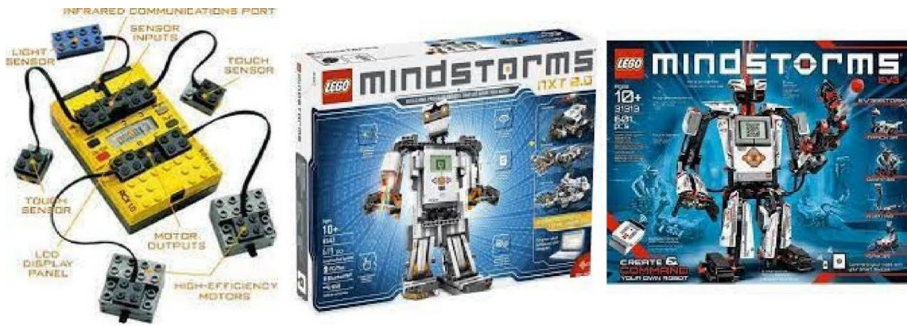
Figure 1-6. LEGO MINDSTORMS series, with the first version, followed by NXT 2.0 and EV3
