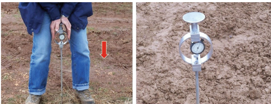
Fig. 2.1 Penetrometer—measurement of the bearing capacity of soil ( Cone Penetrometer , kPa/psi; Soil trafficability )
