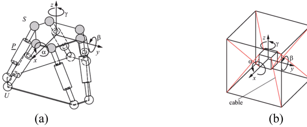
Fig. 1. Robots of parallel structure: a) Stewart parallel robot; b) CDPR
