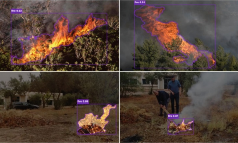
Fig. 4. Segmentation of forest fires: Illustrative examples with YOLOv8.
