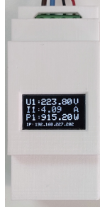
Fig. 4. Consumption Energy Monitor
