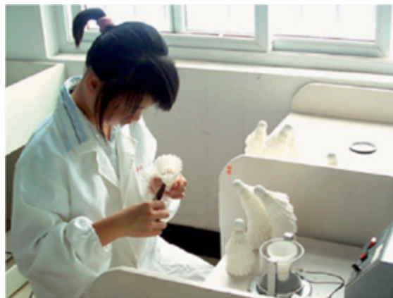
Fig. 8: In the Victor shuttlecock factory in Nanjing in China, the distance between each individual feather is checked by hand.
