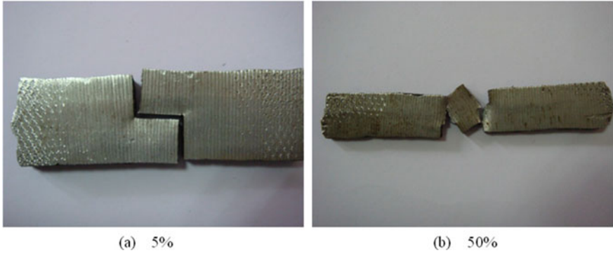
Fig. 2.12 Tensile fracture of roll bonded samples
