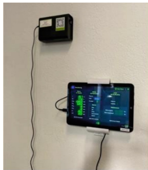
Fig. 1. Sensor for air-quality monitoring (up-left) and Smart Control Display to check air parameters and IoT systems operating (down-right).
