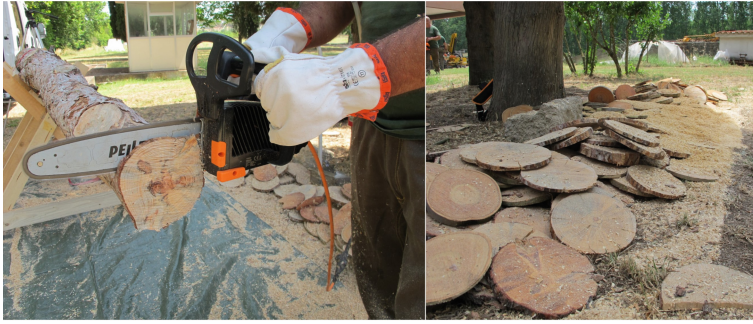
Fig. 1. View of the cutting operations and resulting slices of wood.
