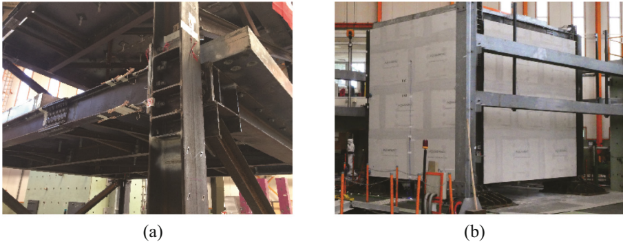
Fig. 7. Examples of the assembled mockups: (a) bare frame with RBS joints, (b) infilled.
