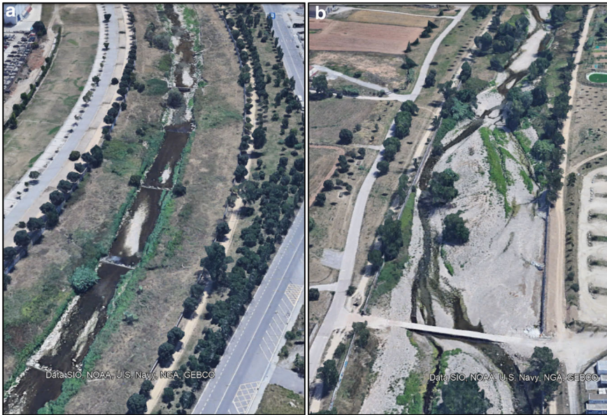
Fig. 1.2 Images of the river Congost (Granollers, Barcelona). In a the river is channelised and immobilised by parallel roads, while in b the hydro-geomorphological processes and the channel's morphology have been recovered following the elimination of these roads. Source Images taken from Google Earth (2021)
