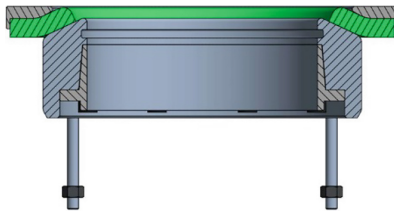
Fig. 2. Section of the mounted seal: in green the ring made in polyester.
