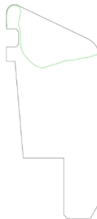
Fig. 6. Unworn profile (black) and final worn profile (green) of metal ring.
