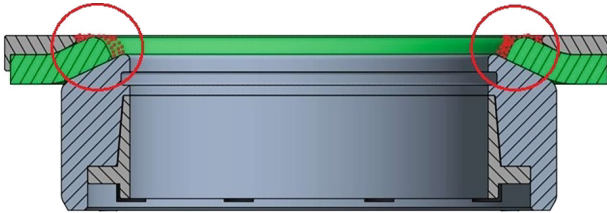
Fig. 8. Concrete particles accumulation zones inside the seal.
