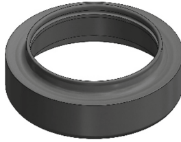
Fig. 5. 3D digital model of the worn metal ring obtained by 3D scanning.
