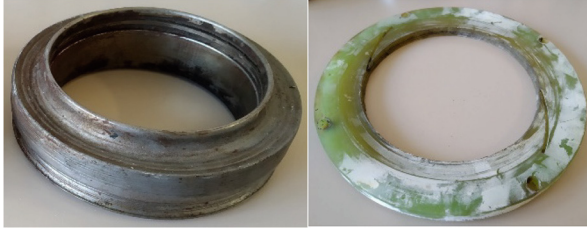
Fig. 3. The worn rings of the mechanical face seal.
