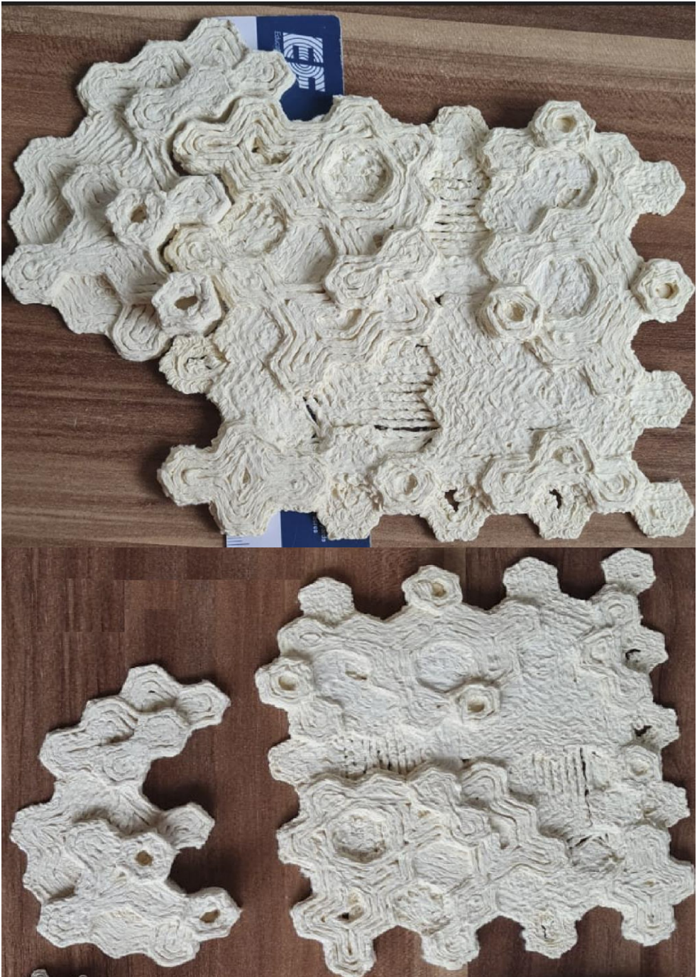
3D paper printed object showing edge details for interlocking.
