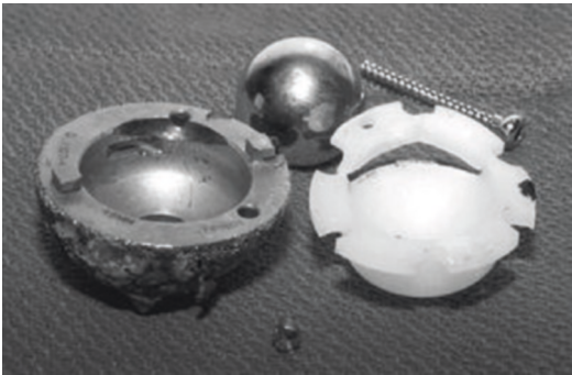
Fig. 2.11 A 1-year conventional UHMWPE, primary acetabular liner demonstrating crack initiation and propagation. Failure initiated at a sharp edge of a locking point (from Tradonsky S, Postak PD, Froimson AI, et al. A comparison of disassociation strength of modular acetabular components. Clin Orthop Relat Res. 1993;296:154–160, with permission)
