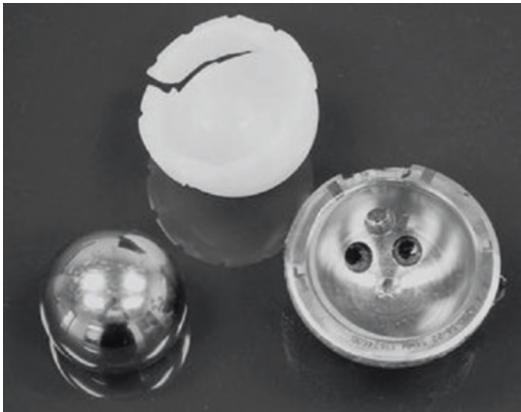
Fig. 2.12 A 10-month cross-linked UHMWPE, revision acetabular liner demonstrating crack initiation and propagation. The decision to retain the acetabular shell in an almost vertical and anteverted position contributed to this early failure, which was compounded by the decision to use a 40-mm femoral head and a correspondingly thin liner (from Halley D, Glassman A, Crowninshield RD. Recurrent dislocation after revision total hip replacement with a large prosthetic femoral head. J Bone Joint Surg Am. 2004;86(4):827–830, with permission)
