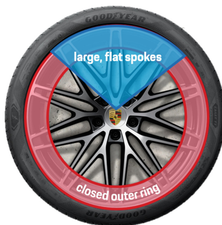
Fig. 12. Aerodynamic rim optimisation
