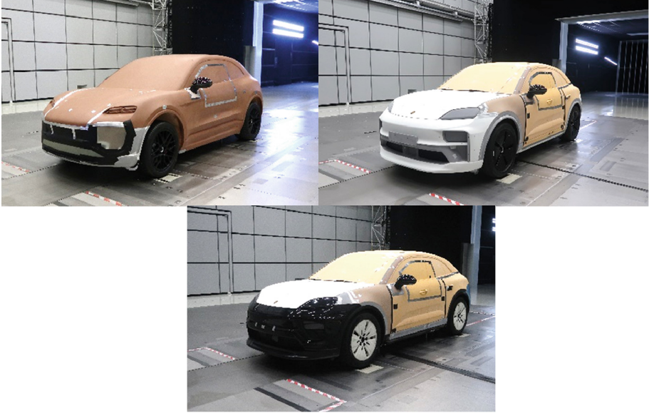
Fig. 4. Evolution of modular aerodynamics model (from left: clay, hard foam, series components)
