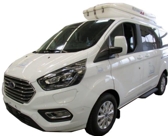
Fig. 13. H 2 ICE Democar (people mover version), already equipped with the fuel storage system on the vehicle roof.
