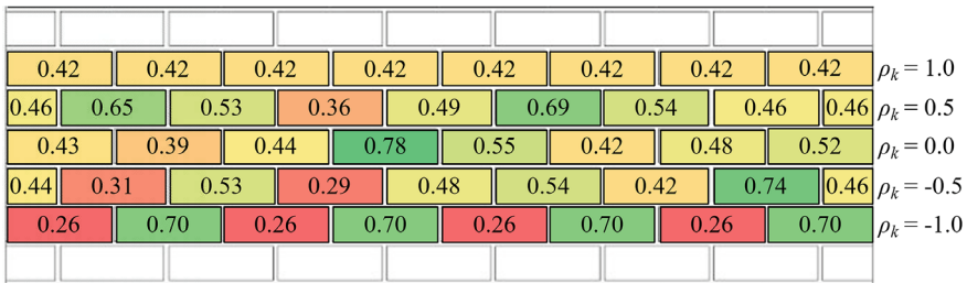
Fig. 1 Indicative flexural bond strengths for various correlation coefficients
