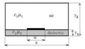
Instead, the propagation along the microstrip line is a function of z and takes place in the form of a progressive wave:
