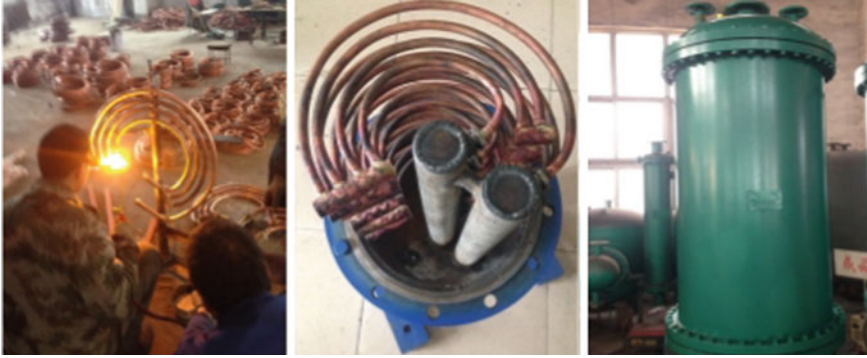
Fig. 1.3 Manufacturing process and finished products of ETB heat exchangers
