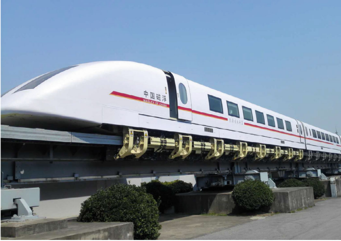
Fig. 1.6 Tongji University high-speed maglev test line and PEM hybrid maglev train
