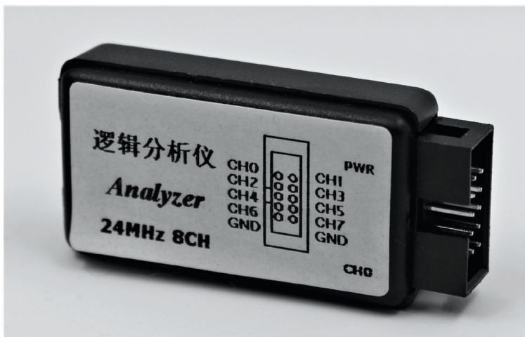
Figure 1.6: An affordable 8-channel Logic Analyzer for getting started with protocol analysis.
