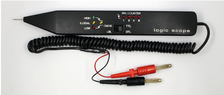
Figure 1.7: A logic scope from the 1980s which can also count in binary.
