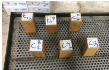
Fig. 3. Control mortar samples being tested for water absorption coefficient.
