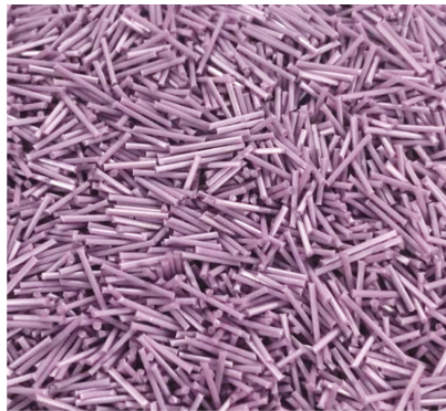
Fig. 1. Short PET fibres with 0.45 mm diameter and 6 mm length.
