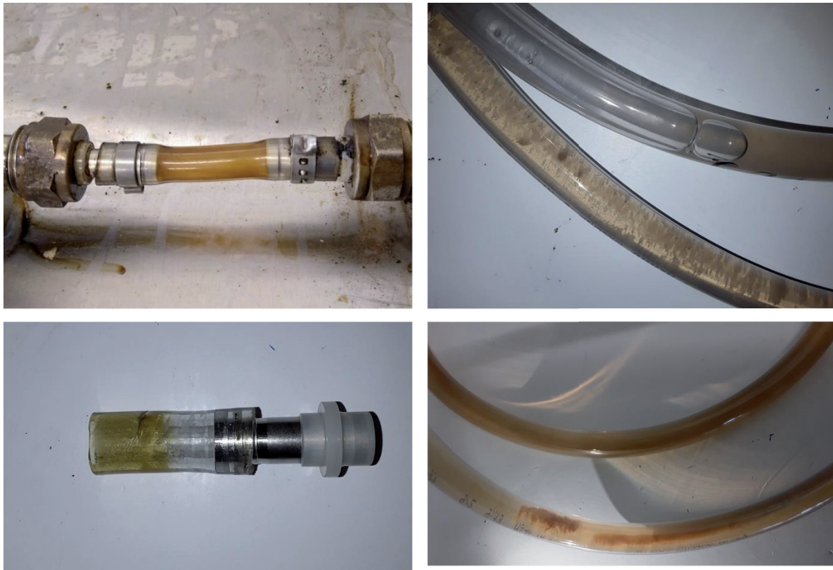
Fig. 1 Exemplary images of spoiled beer transfer tubes showing biofilm formation and fouling on the hose surface with beer contact
