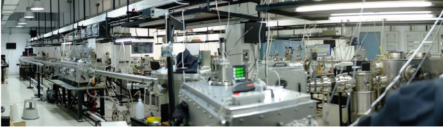
Fig. 1.1 The 18 m long 20GW attosecond beamline of the attosecond science and technology laboratory of FORTH. Attosecond emission is based on high harmonic generation in noble gas media introduced through a dual-pulsed-jet configuration
