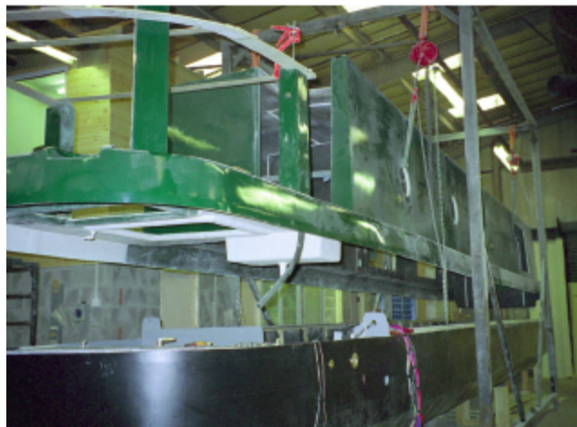
Modern fibreglass 'cruiser' type narrow boat, Zena, under construction in 1997
