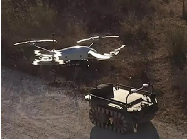
Fig. 3. Heterogeneous cluster composed of Probot unmanned vehicles and “Thor” unmanned aerial vehicles.
