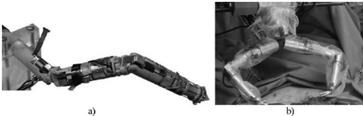
Figure 1.5. Architectures with rigid links and discrete joints: a) DRIMIS (ISIR) [SAL 04]; b) SPRINT (Araknes project) [PIC 10, SAN 11]
