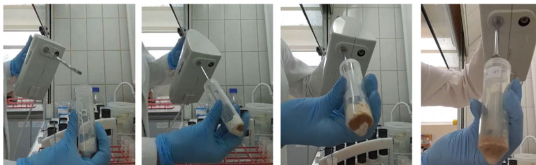
Fig. 3 Utilization of an adapted manual cake mixer with dough hooks to perform the matrix solid-phase dispersion of perlite over a mussel sample
