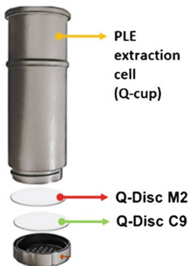
Fig. 1 Positioning of filters in the Q-Cup® tube for use in an EDGE pressurized liquid extraction system for extracting PAHs from fish
