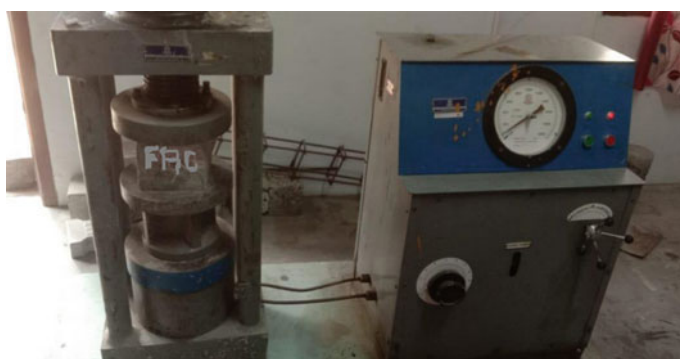
Fig. 1 Compression testing of a cube specimen
