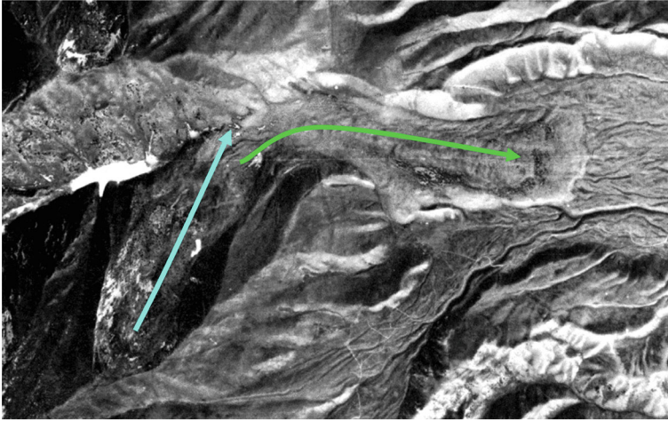
Fig. 1.6 Southern Karakungey secondary RA with almost 90° change of debris motion direction. Blue arrow—direction of the initial slope failure; green arrow—that of the secondary failure
