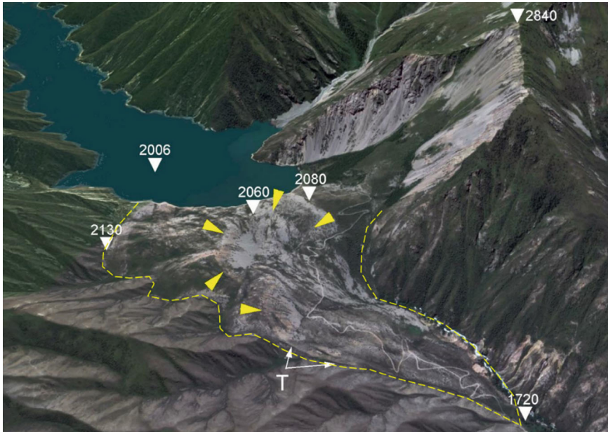
Fig. 1.4 Frontally confined widened Karasu Lake RA of the secondary type described hereafter, Central Tien Shan, Kyrgyzstan. Yellow dashed line—boundary of the dam body; yellow triangles mark the so-called secondary scar; T—trimline of the secondary rock avalanche
