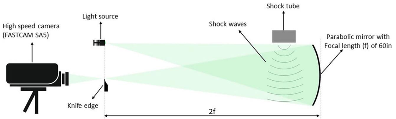
**Fig. 2** Schlieren imaging setup consisting of a 530 nm, 32.5 mW, LED, directed through the volume of interest and reaching a parabolic mirror with a focal length  $f$ . The reflected light is focused at a distance  $2f$ , passing through a knife edge, and detected by a high-speed camera
